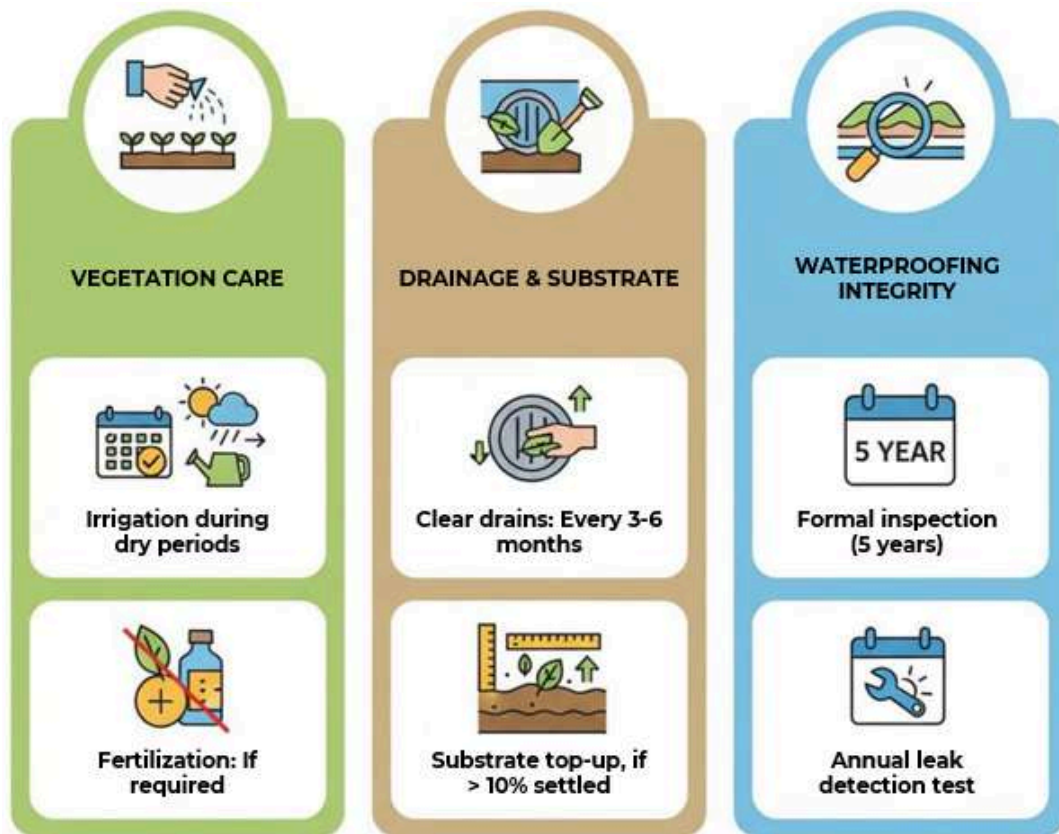
Figure 14 Recommended maintenance schedule for green roofs
