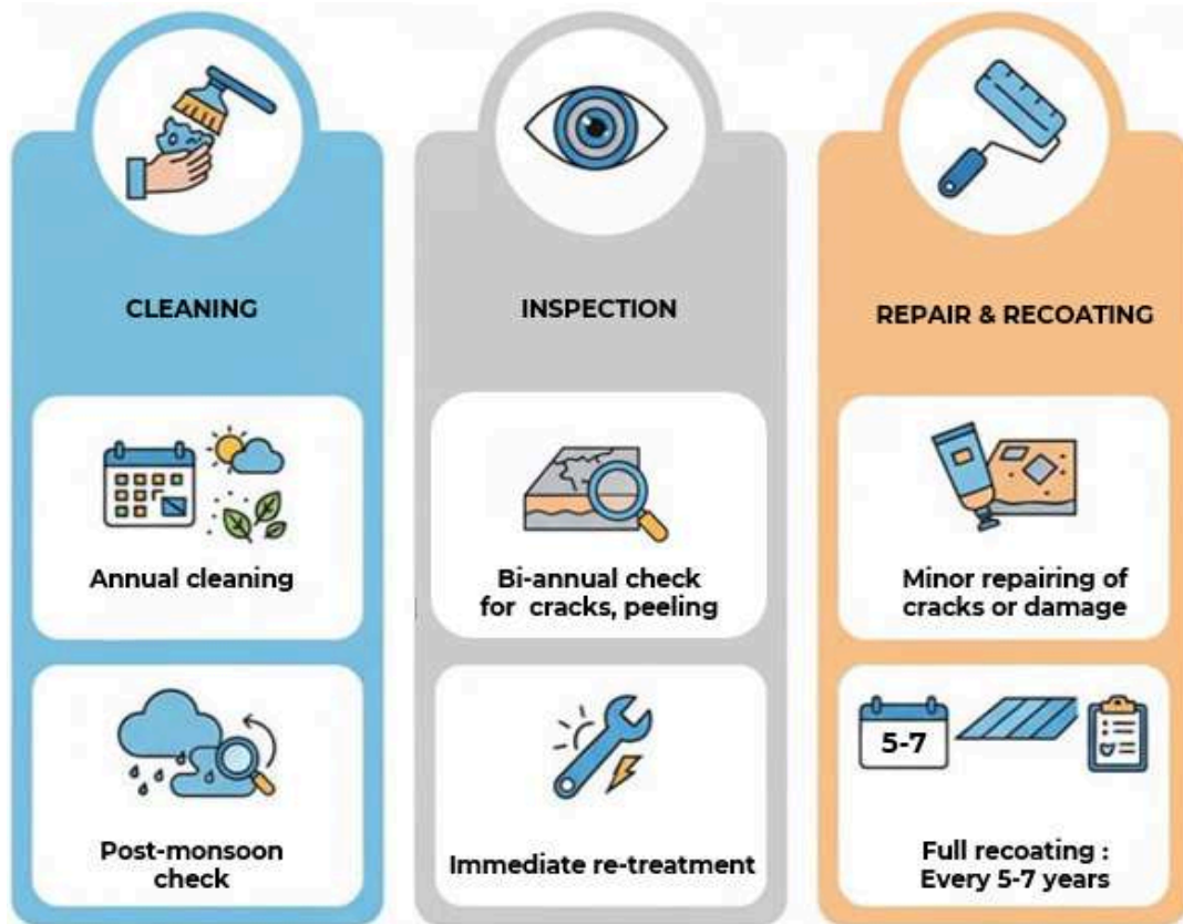
Figure 13 Recommended maintenance schedule for cool roofs
