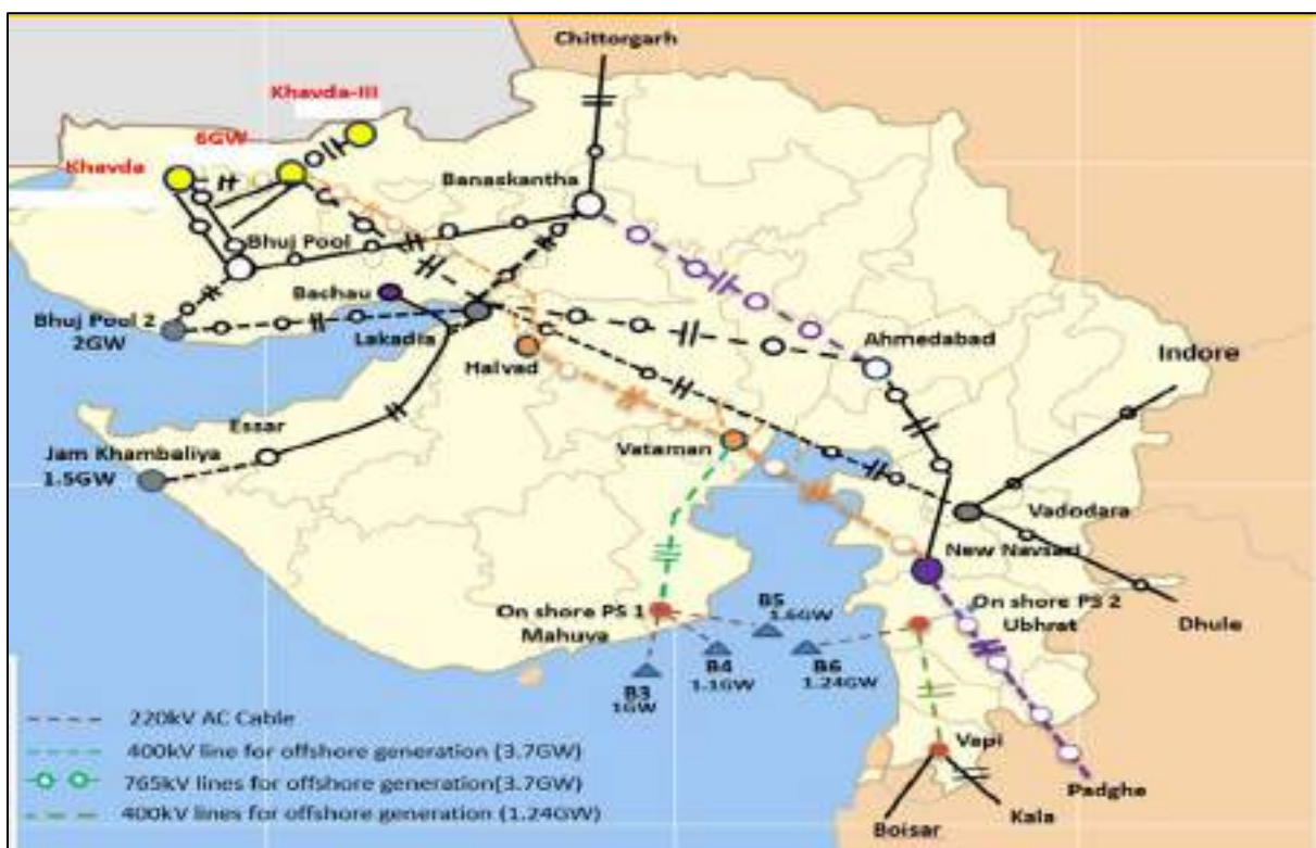
Fig. 10.4: Transmission system for off-shore wind potential zones in Gujarat
