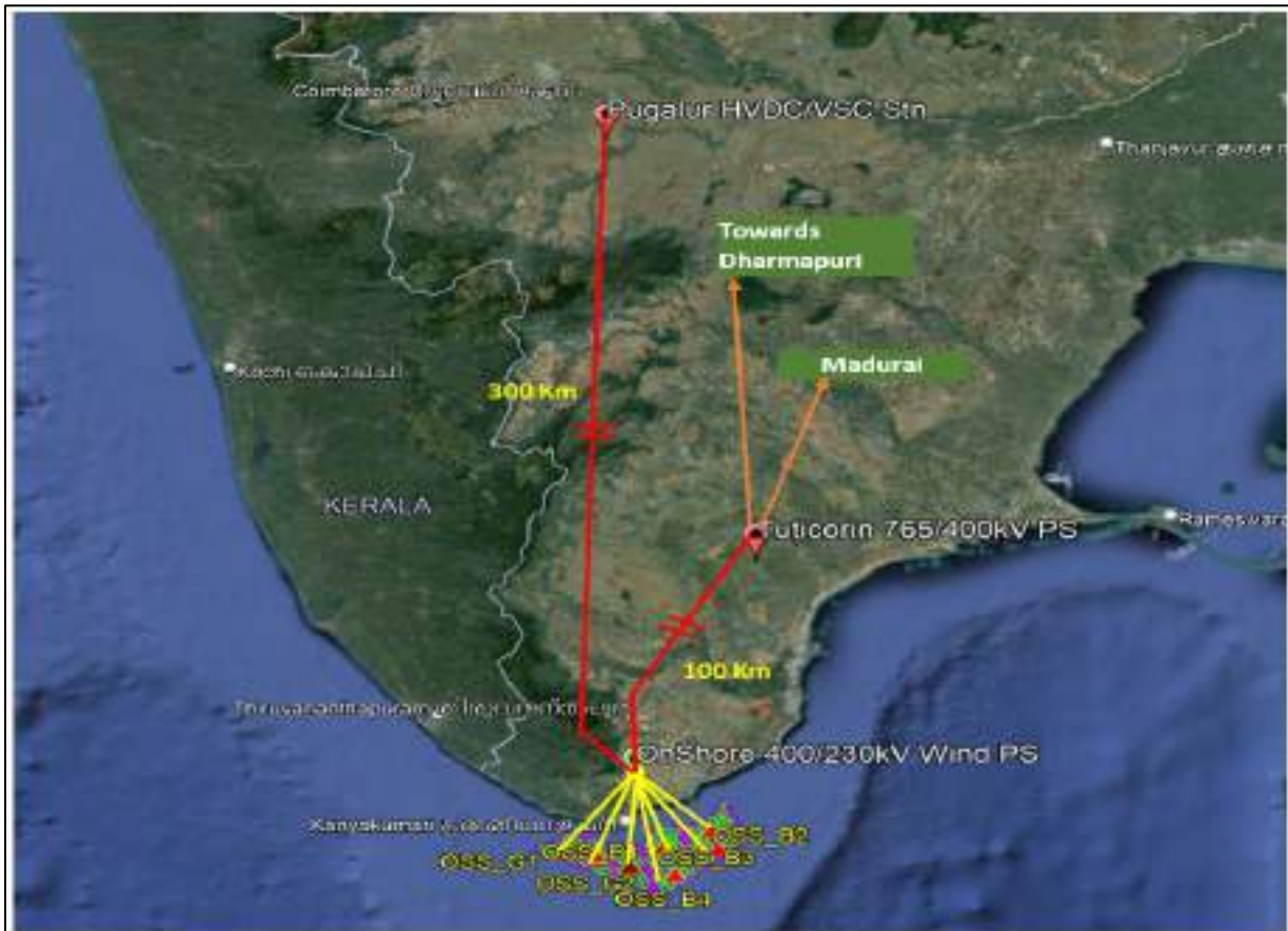
Fig. 10.9: Transmission system for off-shore wind potential zones in Tamil Nadu
