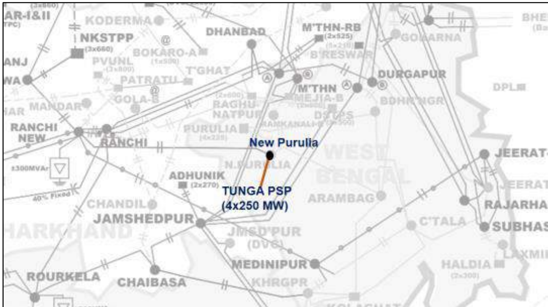
Fig. 11: Transmission system for evacuation of Turga PSP in West Bengal
